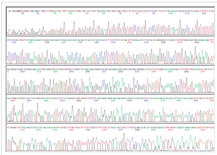
BigDye® Terminator Sequencing Standard run on the ABI Prism® 3100-Avant Genetic Analyzer with POP-6™ polymer.
