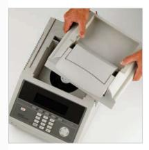
Easily interchangeable sample blocks let you configure the GeneAmp<sup>®</sup> PCR System 9700 for a wide range of PCR and cycle sequencing methods.
